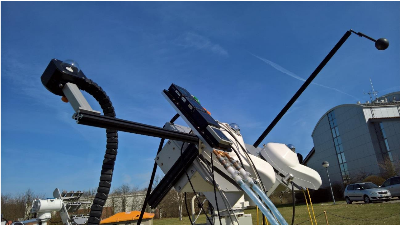
Figure 9: Picture of the new outdoor facility. In the centre of the picture you can see the solar cells mounted on a two axis sun tracker. The solar cells are mounted on water cooled Peltier elements. On the left-hand side, a cosine-corrected probe is mounted for three spectroradiometers, which uses the data from the sky scanner.
