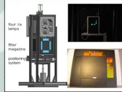
Fig. 1(b) Pulsed solar simulator used as a light source with narrowband filters (SUPSI) [2].
