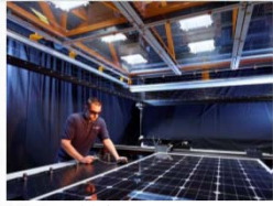
Fig. 1(a) Spectral response measurement apparatus at TUV [1].
