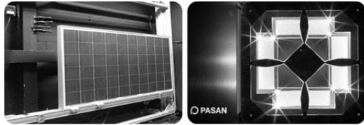
Fig. 1 Image of light bulbs (right) and measurement rig (left) of the solar simulator used.
