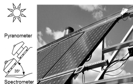
Fig. 7 Outdoor PV performance and meteorological data monitoring system.
