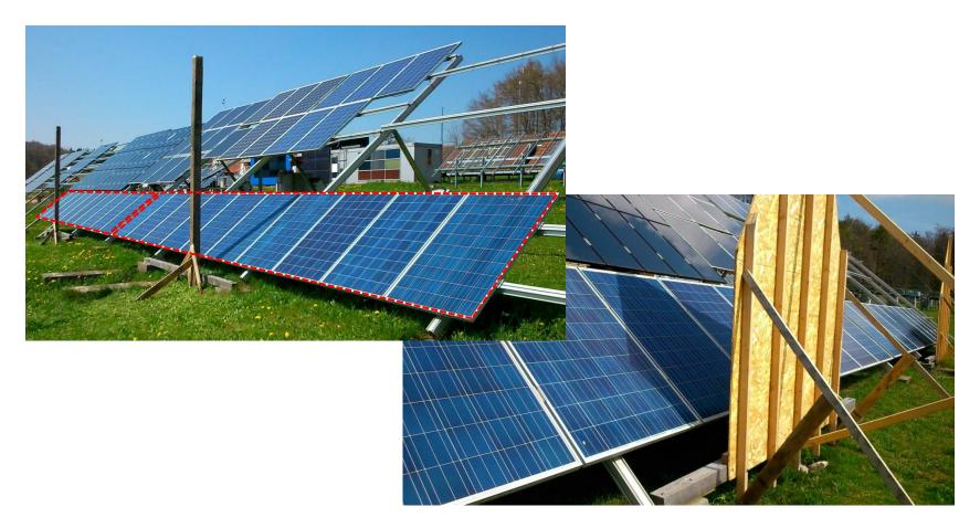
• 'pole' shading and 'gable wall' shading configuration
