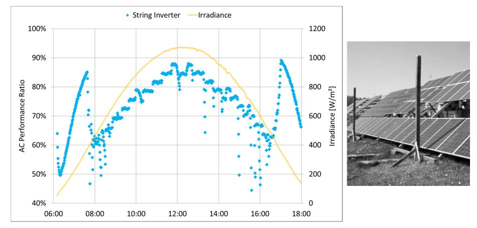
performance steps according to module substrings affected by the shadow
