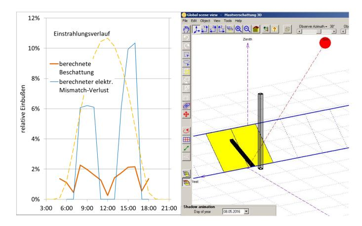
computed shading effect drops strongly around noon although shadow is continuously present
